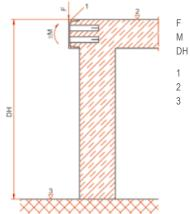
Transverse force 84 kN Bending moment (kNm) Ramp height U 200 DIN 1026 Ramp
