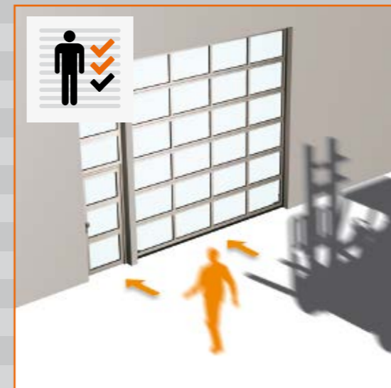
Separate doors for pedestrians and goods, but in the same opening structure.
