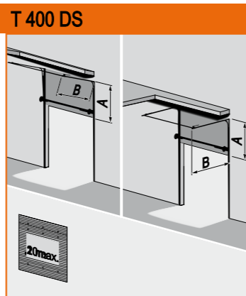
T 400 DS Elevated rail system with low spring axis
