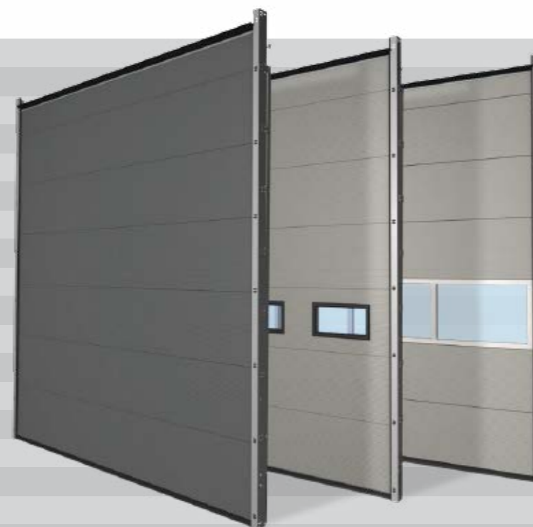
U-value ISO 60 mm sectional door: 5,000 x 5,000 mm: 0.84 W/m 2 K
