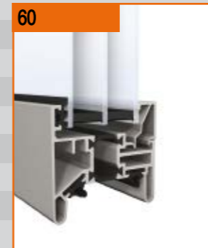
NOV661 60 mm Triple Plexiglas Optical 40 mm (4-14.75-2.5-14.75-4 mm)
